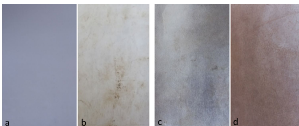
Fig. 7 NADIR® UP150 T membrane samples a : non-modified, b : coated 45% intensity, c : coated 95% intensity, d : coated 66% intensity (default)
